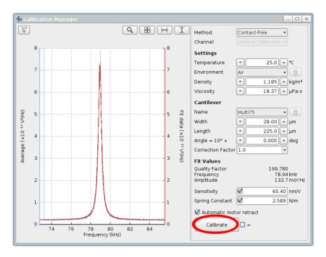
If the calibration fails. If it does not fit a peak within your cantilever's frequency range. You will need to manually select a peak. There should be a clear peak in the spectrum, within your cantilever's stated frequency range. It should be similar to below. If not see troubleshooting, in the Appendix.
