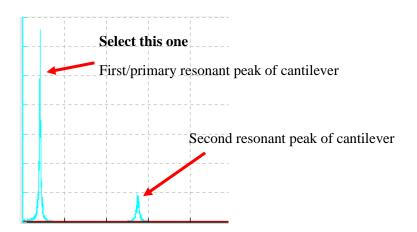
To manually fit a peak select the icon on the top left corner of the window. Click and drag the cursor horizontally over peak area in the spectrum window. This should select the peak. If not try a wider region before and after the peak. If this does not work, you may need to try a different calibration technique. Consult the general set-up manual.
