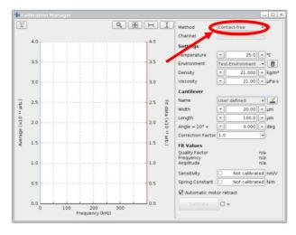
(c) Set the Environment to 'Air'. The density and viscosity are prefilled but can be altered.
