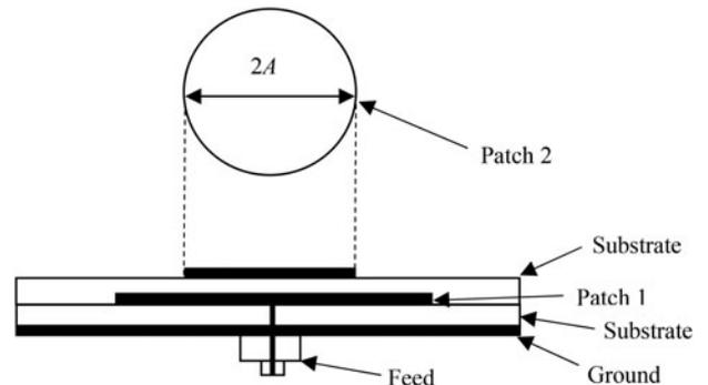
Fig. 2. Cross-sectional view of single-feed stacked microstrip antenna.
