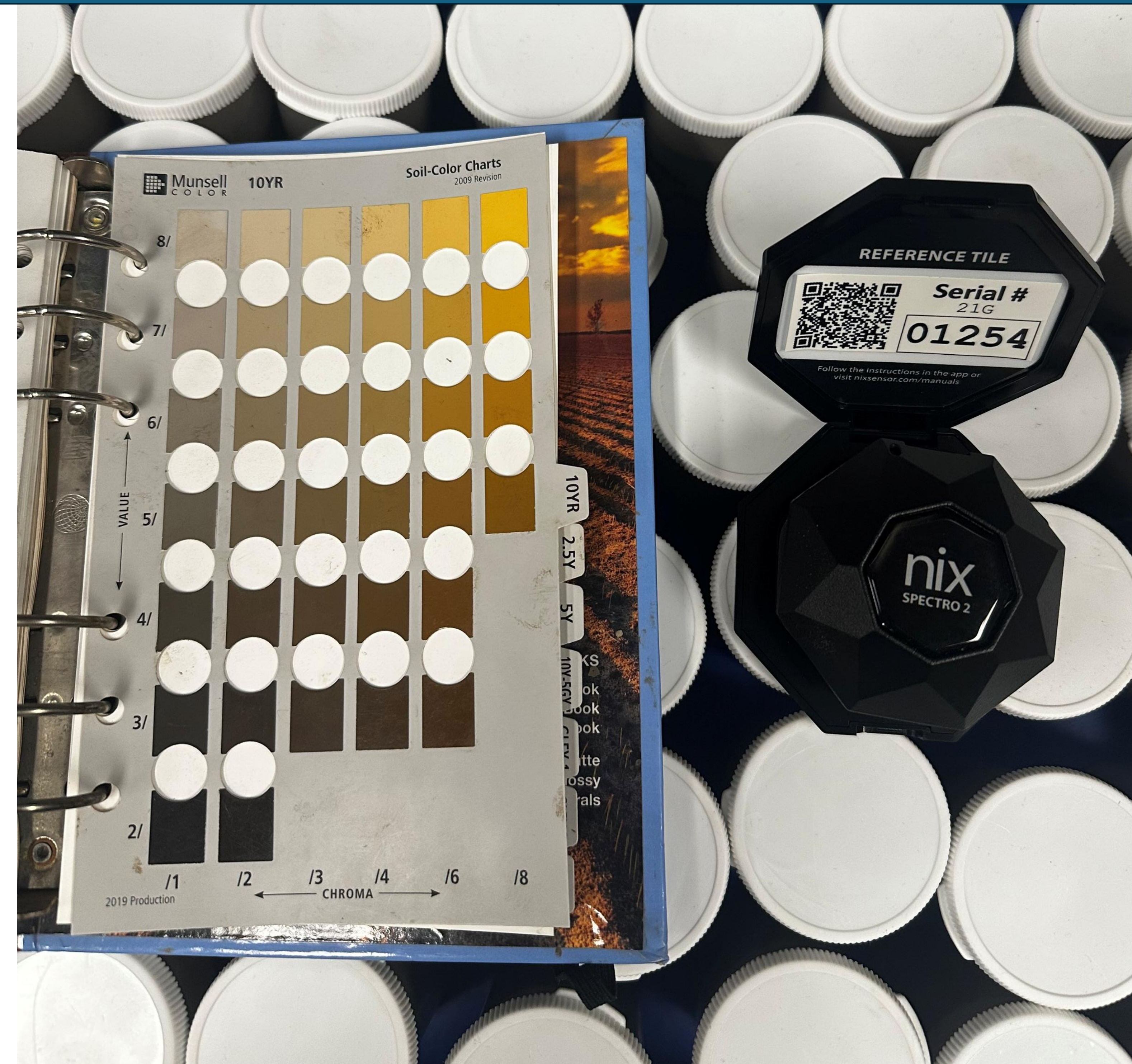
Figure 3. Munsell guide opened to page 10YR and NIX Spectro 2 sensor on top of various soil sample vials.
