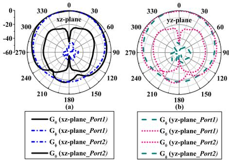
Fig. 3. Simulated normalized radiation pattern of the proposed MIMO DRA (a) xz-plane (b) yz-plane
