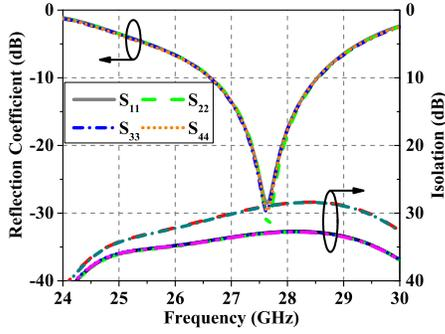
Fig. 2. Simulated response of the MIMO DRA
