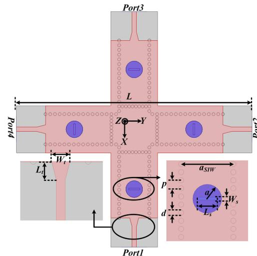
Fig. 1. Schematic of proposed SIW fed MIMO DRA.  $L = 35.04$ ,  $L_t = 1.32$ ,  $W_t = 1.32$ ,  $p = 0.7$ ,  $d = 0.455$ ,  $a_{SIW} = 4.5$ ,  $a = 1.25$ ,  $L_s = 1.65$ ,  $W_s = 0.25$  (all dimensions are in mm)
