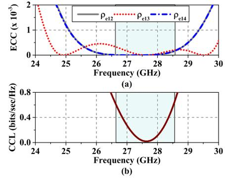
Fig. 4. Simulated variation of (a) ECC (b) channel capacity loss with frequency
