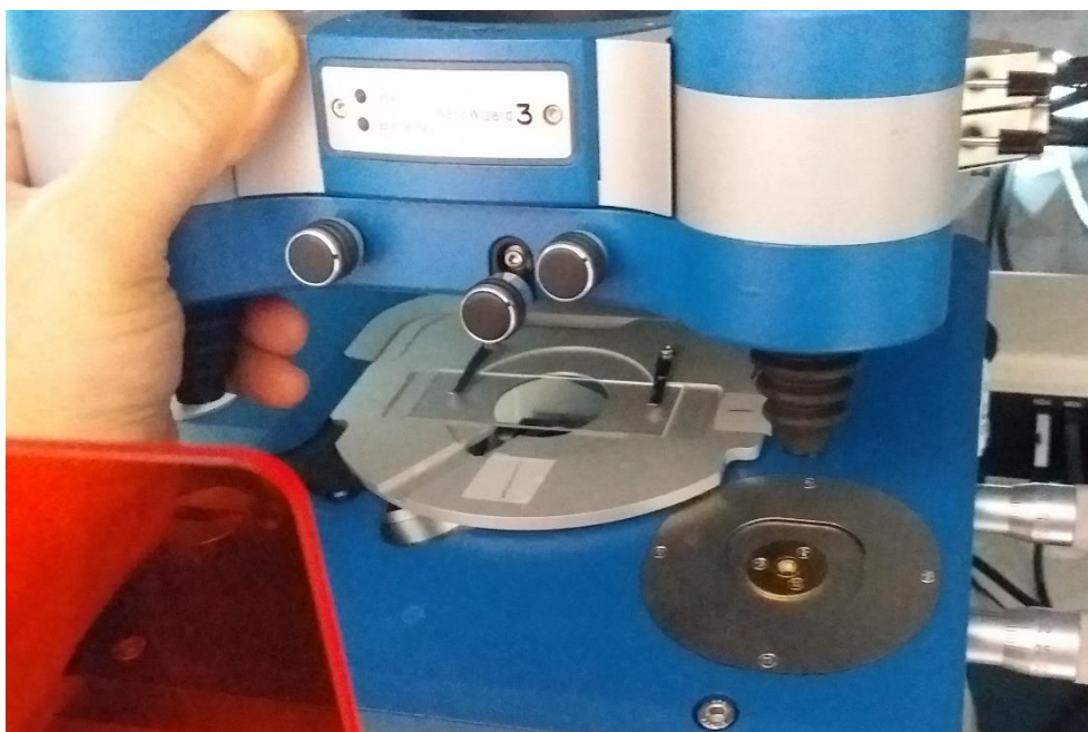
Figure 9: Place the AFM Head Unit rear leg down before the two front legs.
