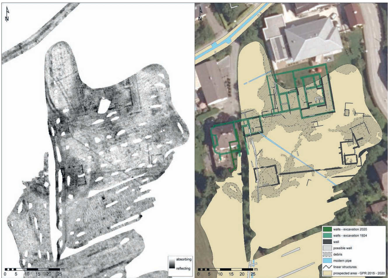
Figure 2. Roman villa of Weyregg. Left: GPR time slice (depth 0.40–1.40 m), right: archaeological interpretative map of the survey data.
