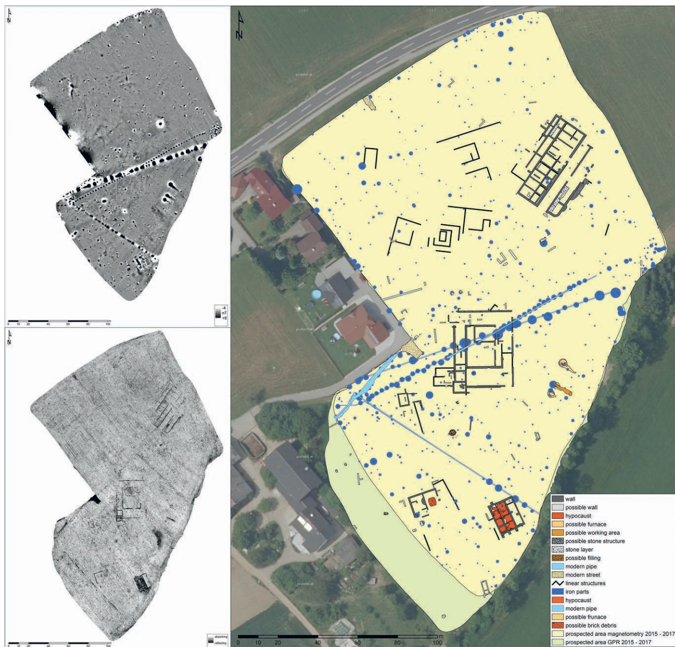
Figure 1. Villa rustica of Königswiesen. Top left: Magnetogram (-4/+6 nT), bottom left: GPR time slice (depth 0.25–1.20 m), right: archaeological interpretative map of the survey data.
