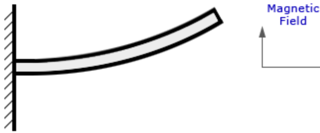
Figure 4: Magnetised MFM cantilever.
