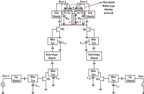
Fig. 3: Schematic of cascade differential LNA with marchand balun type biasing network.
