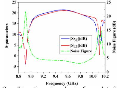
Fig. 5: Overall insertion gain and noise figure plot of the rat-race hybrid fed differential LNA.
