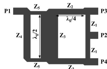
Fig. 2: Layout of the two section rat-race hybrid.
