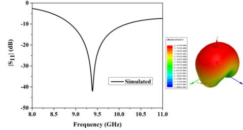
Fig. 6: Simulated  $S_{11}$  and 3D radiation pattern (9.5 GHz).
