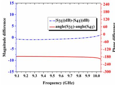
Fig. 4: Magnitude and phase difference of hybrid outputs.
