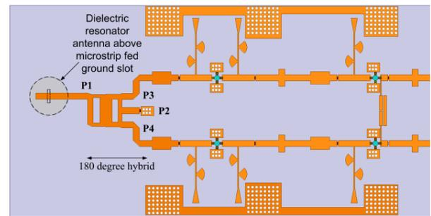
Fig. 1: Layout of the amplifier antenna.
